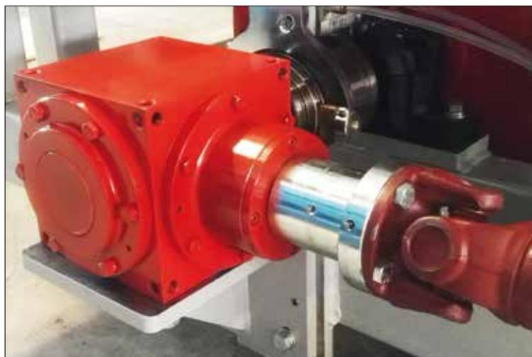
**DIRECT MECHANICAL CONNECTION,** to faithfully replicate the road working conditions. The front-rear connection is 'excludable', a peculiar feature of Dimsport Dynorace power bench testers.
