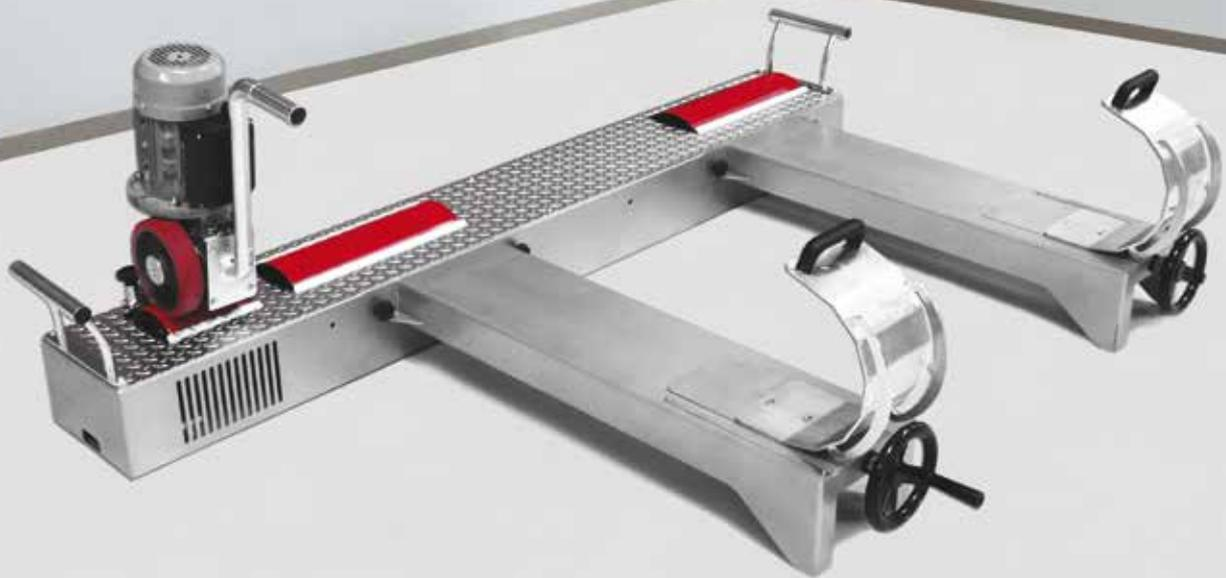
Dyno Kart is a chassis dynamometer developed to measure torque and power (up to 100 hp) delivered at the wheel for karts provided with or without gearbox. Thanks to a dedicated and specifically conceived eddy current brake, Dyno Kart allows to **perform tests with load simulation on 60-100-125 cc highly performing karts**, in addition to the regular acceleration tests.
