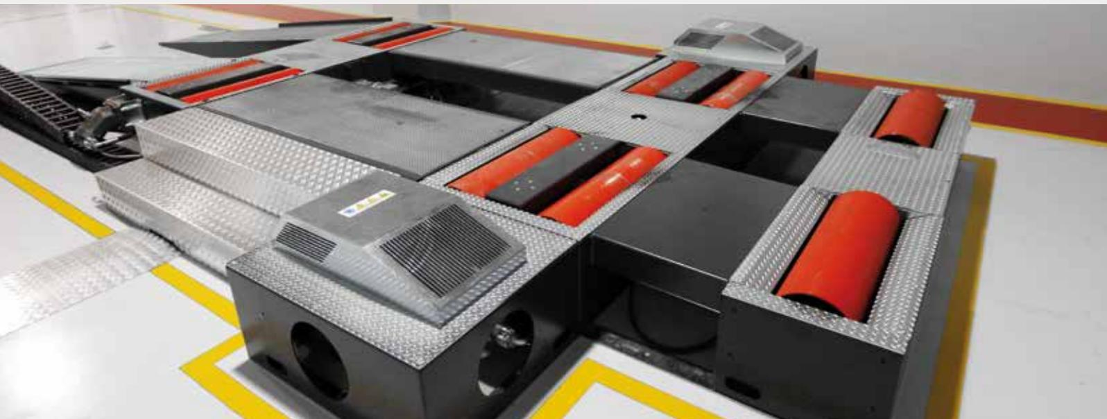
Dynotruck represents Dimsport's offer for power test and road simulation of **heavy duty vehicles**. Targets are **test of vehicle working, dynamic diagnosis** and **engine parameters tuning**.
