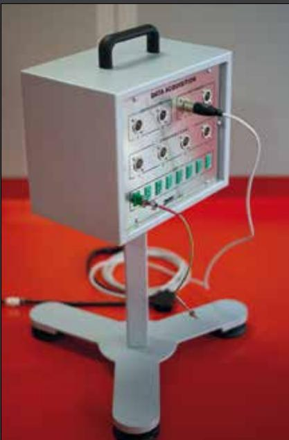
Data acquisition box to accommodate a total of 8 exhaust gas temperature probes, 2 oxygen probes, 2 turbo pressure probes and 4 additional configurable inputs
