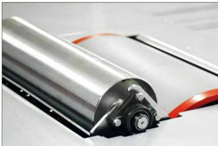
**POSITIONING ROLLERS** to set the most suitable position (automatically determined by the software by inputting the tire size) and also to identify situations of slip between tire and roller.
