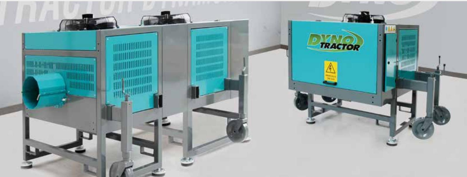
Dyno Tractor is a **diagnostic system developed for agricultural vehicles provided with cardan shaft.**
