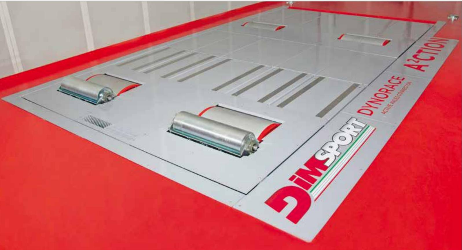
The new Dynorace **A<sup>2</sup>CTION** power bench tester has been designed and developed to support the latest vehicles technology: the result is extraordinary, a **4WD braked dynamometer, provided with SINGLE ROLLER FRAME** and **rigid connection between front and rear axle** (thanks to a **driveshaft**).
